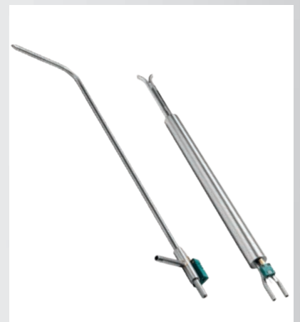
Gas flow velocity measurement (m/s) by means of pitot tubes
