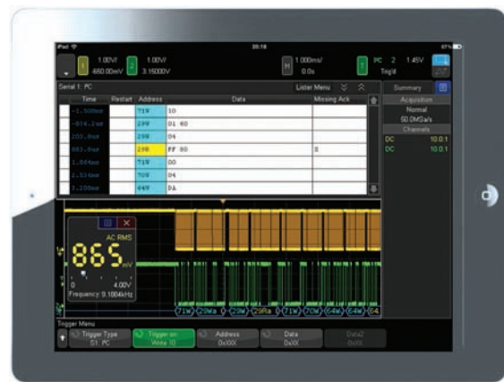
Figure 38. Tablet virtual front panel control.
