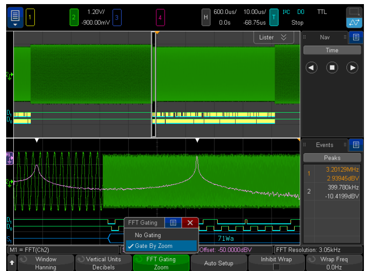
Figure 18. Gated FFT successfully correlated the hopping of the FSK modulation with the analog and I 2 C control command.
