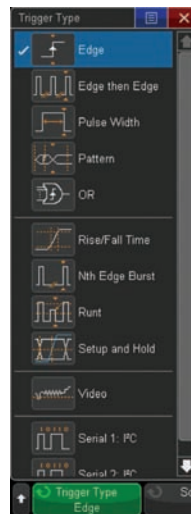
Figure 43. Wide array of advanced parametric trigger modes.
