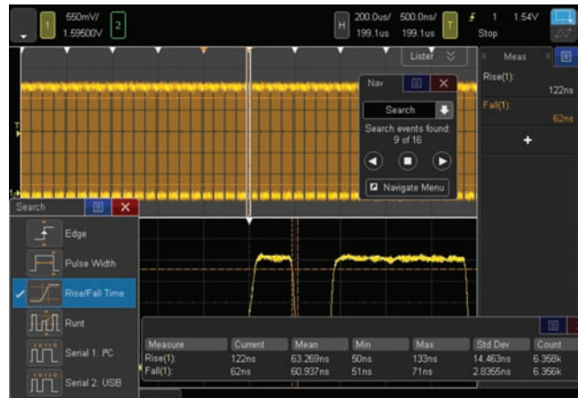
Figure 10a. The 4000 X-Series was set up to capture data signals with various rise time edges. Using the search and navigation capability, the oscilloscope was able to find, mark (white triangles), and quickly navigate to 16 occurrences of "out of compliance" rise-time edges.
