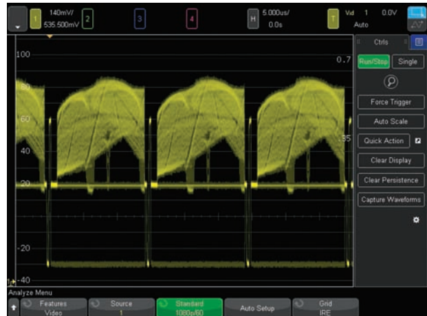
Figure 27. Triggering on 1080p HDTV signal analysis.
