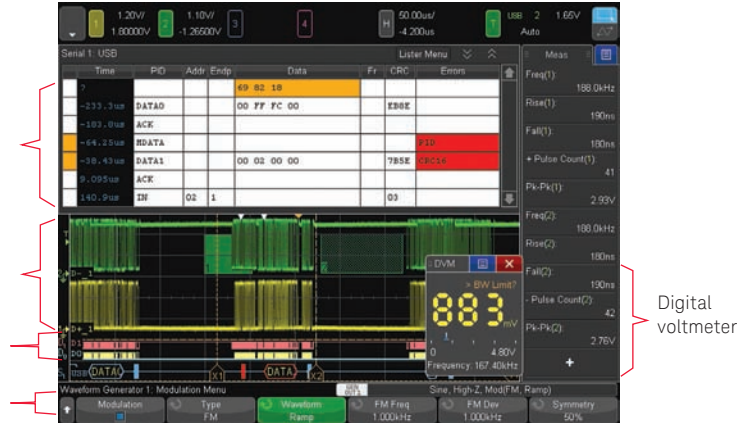
Figure 17. The 4000 X-Series provides the capabilities of five instruments seamlessly integrated into one.
