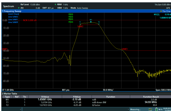
Measurement and qualification of a SAW filter (n-dB down BW, Q-Factor)
