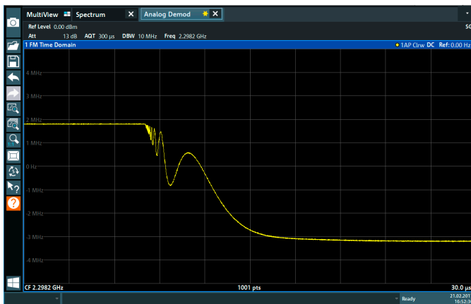
Frequency settling behavior of an oscillator
