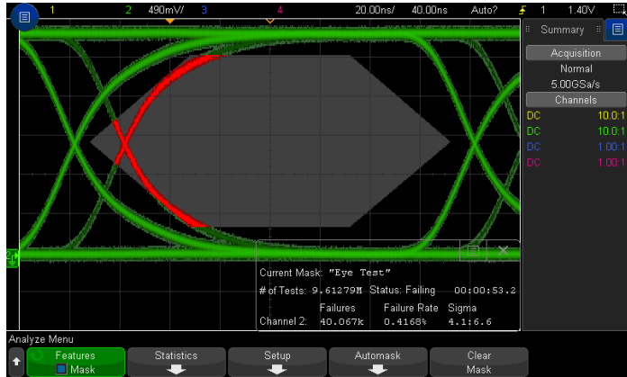
Figure 28. Hardware accelerated mask testing allows testing against a golden waveform or user created mask to find violations. In this example we captured over 5M tests in only 30 seconds.
