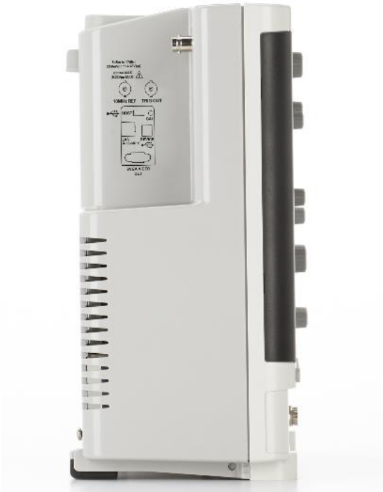
Figure 8. One-gigahertz-per-inch form factor: 6 GHz, 6 inches deep.
