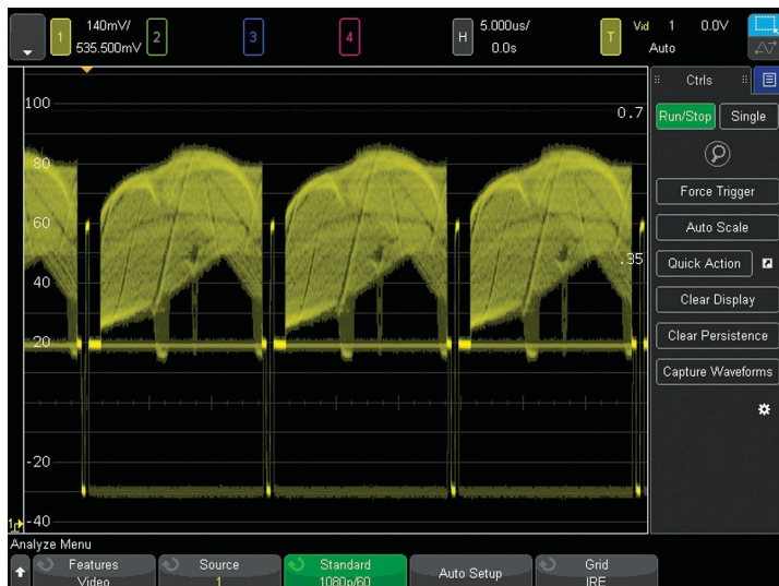
Figure 27. Triggering on 1080p HDTV signal analysis.
