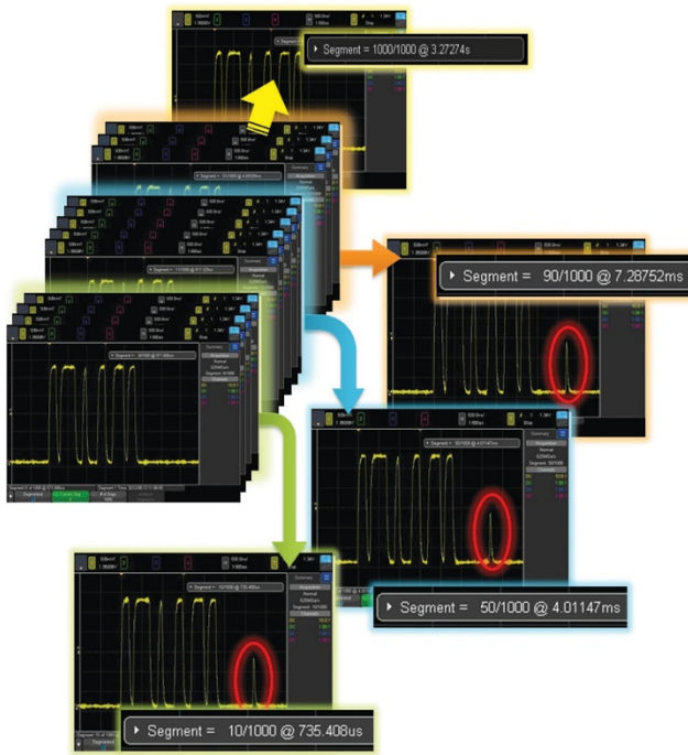
Figure 7. Segmented memory efficiently manages the memory to capture up to 1,000 segments of interest to you, making it an effective ultra-deep memory oscilloscope that can easily capture infrequent events and anomalies.
