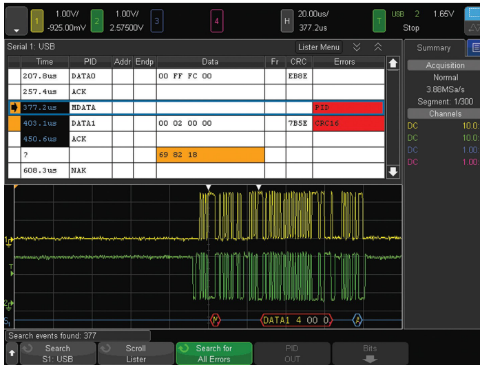
Figure 21. USB 2.0 trigger, decode and “lister” display.
