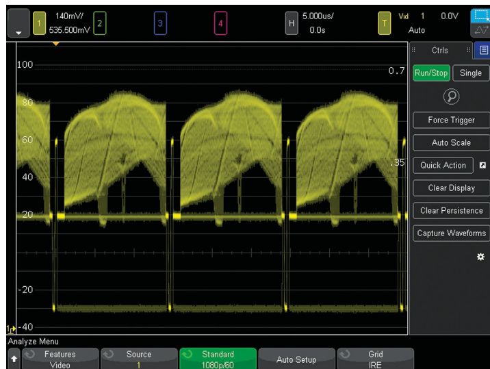
Figure 27. Triggering on 1080p HDTV signal analysis.
